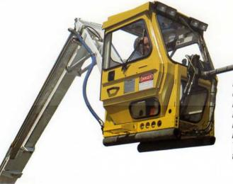
FMC's Enclosed Cabin Option frees deicing operators from the hazards of harsh weather and fluid sprayback -- in a simple, user-friendly design that matches or surpasses all the operational benefits of any unit available.
