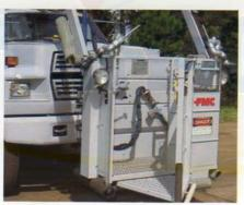
**Ground-level-entry basket** features proportional boom controls for smooth movement and increased operator comfort and safety.
